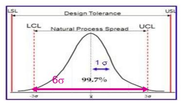
➤ The recommended minimum sample size to calculate Cp is 30 parts
