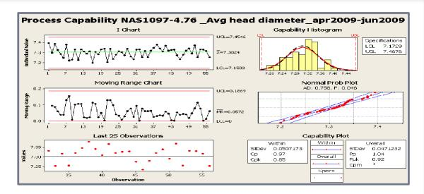
Take into account for the Cp, Cpk calculation all measurements coming from all machines qualified to perform the process step
