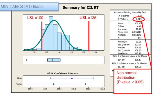
• If the distribution is non-normal, try to understand the root cause of the non normality and/or applied statistical transformation to recover it.
